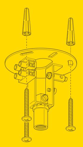
Make earth connection to brass earth terminal and electrical connections to terminal block. Refer to wiring diagram.
