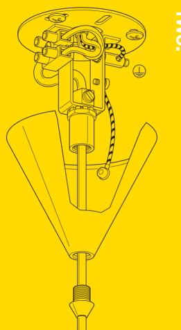
Push cone cover against ceiling and secure with conical screw.
