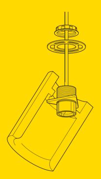
Insert triangular support into shade by tipping at an angle. Raise shade above support to enable easier fitting of the LED lamp. Ensure shade is firmly held when fitting lamp.
